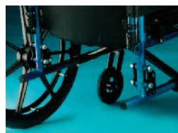
9000 XT wheelchair with offset axle and adjustable angle caster will allow additional seat-to-floor heights and increase seating and positioning capabilities. Offset axle offers center-of-gravity adjustment which increases maneuverability and stability.
